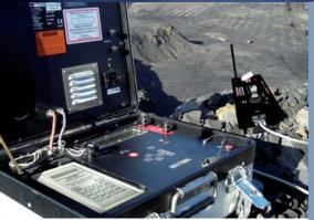
After successful field evaluations in large open-pit operations, Davey Bickford announces the introduction of the Daveytronic® **Wireless Blasting System.** The new system allows technicians to remotely detonate single or multiple shots from a distance of up to 1.5 mile (2.4 km) away from the pattern, significantly improving **safety** during the blast and exceeding minimum distance requirements.
